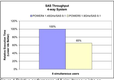
Figure 4 Relative performance of 8 simultaneous jobs on POWER4 and POWER5
