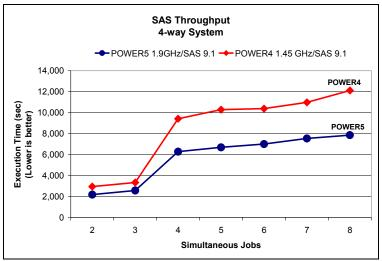
Figure 5 Scaling of SAS 9.1 on IBM POWER processors
