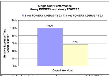
Figure 3 SAS 9.1 single user performance test on POWER4 and POWER5
